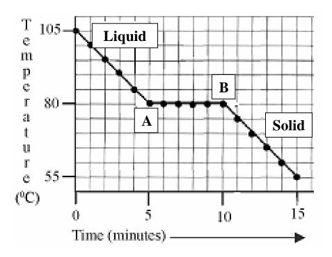
The substance used in this experiment was naphthalene. Naphthalene has a melting point of 80 °C.
