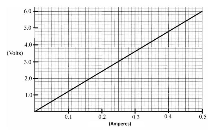
Use this graph to *calculate the resistance* of resistor **R** shown in the diagram. Give the unit of resistance with your answer. (9)
