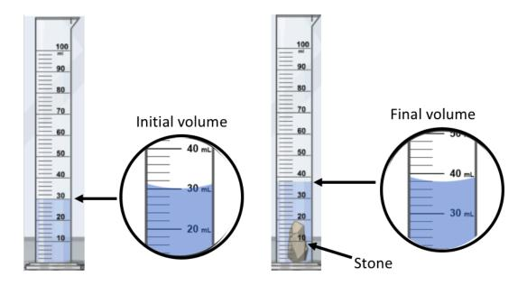
Study the diagram above for measuring the volume of the stone carefully.
